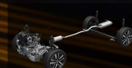
MacPherson Strut & H-Shape Torsion Beam Suspension
